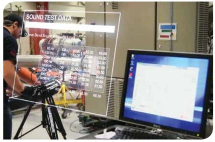
Each CenTraVac chiller is custom-built individually, following rigorous quality control processes. Before a CenTraVac leaves our manufacturing facility, you as a Trane customer can take advantage of our fully customizable portfolio of myTest™ chiller test packages and proof-of-performance options. We invite you to witness all testing before your chiller ships — either in person at our La Crosse, Wisconsin, factory or remotely from the comfort of your office.
